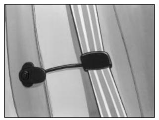
3. Be sure that the belt is not twisted and it lies flat. The elastic cord must be under the belt and the guide on top.
